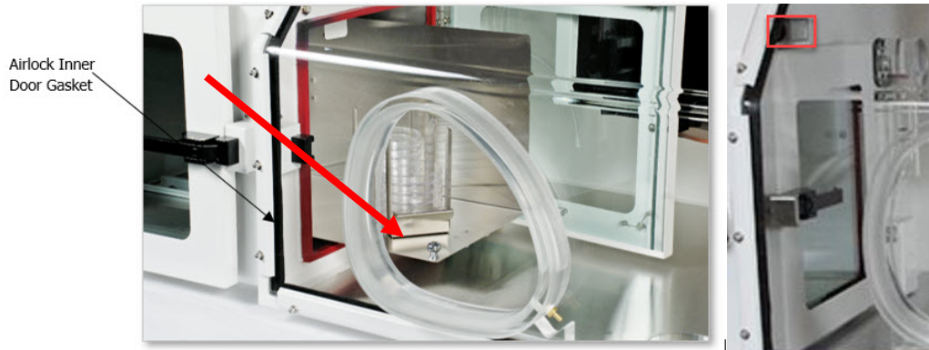
Figure 4: Airlock Inner Door, Sliding Shelf, and Data Plate
